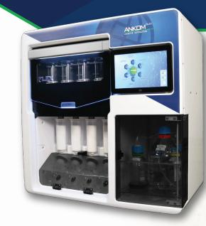
The ANKOM<sup>FLEX</sup> Analyte Extractor is designed to simplify fat-soluble vitamin, cholesterol, and crude and hydrolysis fat determinations. Supporting up to four samples at a time, the system will automatically complete digestion, solid phase extraction (SPE) and evaporation in about two hours.
