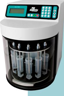
A typical run time of six samples is complete in seconds and with a maximum ability to process six samples per cycle. Up to 300 samples can be homogenized per hour!
